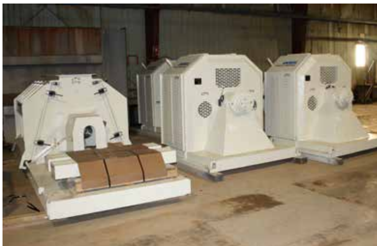
Biomass fuel pellet mills used to produce fuel for Atikokan Generating Station
