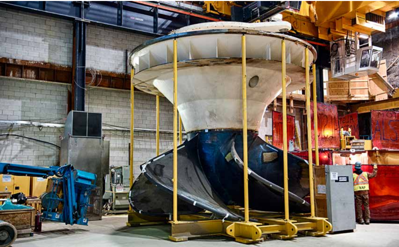
Runner for installation at the new Smoky Falls Generating Station
